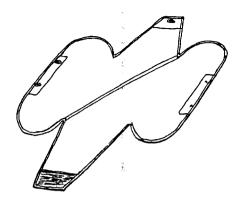
II.) Fold the protruding lines and the bridle on top of the inner container. Turn the inner container over and lay it on top of the outer container so that the bridle loop now protrudes from under the inner container and out of the upper right-hand corner of the outer container, and the double emergency handle lies centrally and evenly on the top of the inner container.
