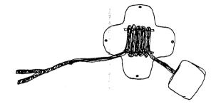
10) Bring the flaps of the inner container over the folded parachute and lines. Insert the loop of lines into the rubber loop of inner container as shown.
