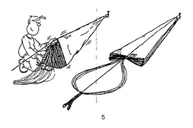
3) Bring the flipped gores back one by one, inspecting them carefully on both sides for wear, damage, stains, deterioration, mildew, etc.
