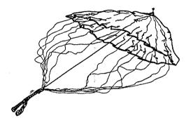
2) Passing a length of the line or strap under all the top lines, including the central line, attach the top to the anchor point.
