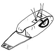
VI.) Lock the loop with the curved pin of the emergency handle. Repeat, in the same order, for the second eyelet and loop.
